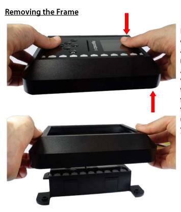
Remove the outer frame to access the mounting plate. Apply pressure with your thumbs on the face and pull the frame upwards with your fingers.
