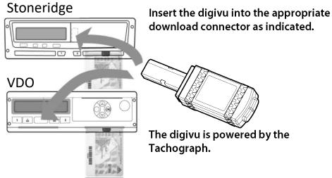
Please note: The new Smart Tachographs vary from the above and therefore download sockets will be located in a slightly different position.
