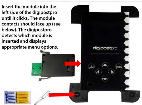
There are four screw points in the base. Use the fixing kit supplied to attach the digipostpro to the wall.
